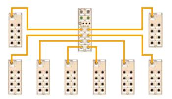
Each IO-Link I/O Hub, directly connected to the IO-Link Master, collects up to 16 standard digital signals on one end and transmits the signals to the controller via the IO-Link system.
